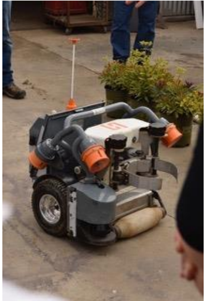
Robot demo at Altman Plants. The robot is used to move plants around the warehouse floor.
